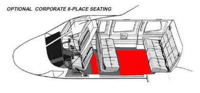
Corporate 8-Place Seating - Six deep bolstered fine wool fabric covered high-backed seats, arranged with one row of three facing rearward, and one row of three facing forward. The optional corporate trim complements the corporate seating and includes: Floor covered with tightly woven wool carpet; side wall armrests, and decorative accent fabric covering for the aft cabin bulkhead.
