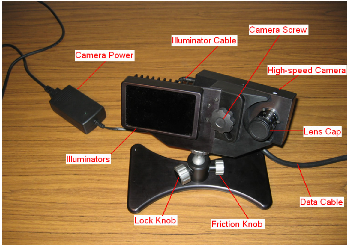
Figure 3-5: Parts of the EyeLink 1000 Desktop Mount
