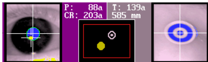
Figure 3-15. Target and Eye Positions in the Thumbnail Camera Images
