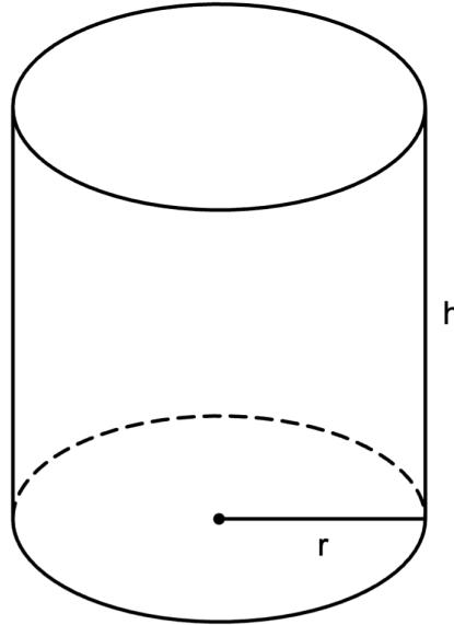
Here,  $r$  is the radius of the base of the cylinder and  $h$  is its height, both in inches. Also let  $V$  be the volume, in cubic inches, and let  $A$  be the area of the top and side combined, in square inches. The bottom has area  $\pi r^2$ . The side, if cut vertically and rolled out flat, is a rectangle with one side of length  $h$  and the other of length  $2\pi r$  (the circumference of the circle). Therefore the relations are
