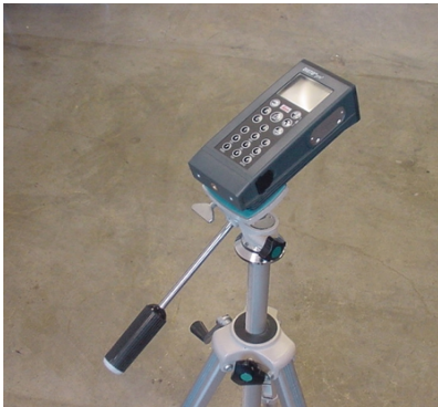
Incorrect attachment to tripod
