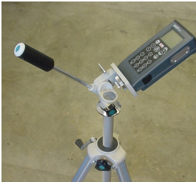
Correct attachment to tripod. Adapter end cover attaches the Disto to the tripod
