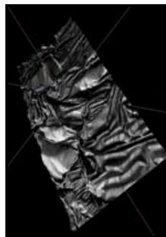
Reconstructed digital elevation model (DEM) of wrinkled glass surface at 500 x, using stereo imaging in the SEM
