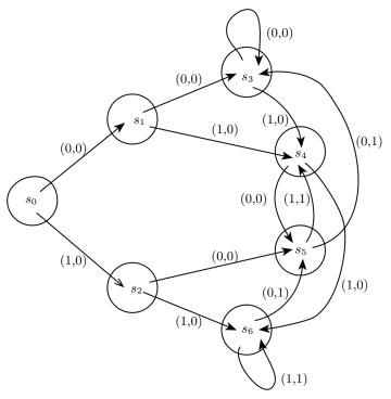
We notice that the states  $s_0, s_1, s_2$  have only 0 as an output, and the states  $s_3, s_4, s_5, s_6$  "remember" the prior inputs 00, 10, 10, 11 respectively.
