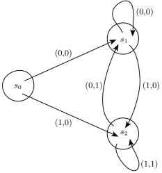
The case k = 2 is essentially more complicated since the machine has to remember two previous digits. Here the input sequence 11110111101110110... gives the output 00111101110110110... Here is the diagram describing the functions  $\nu$  and  $\omega$ :
