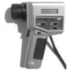
Fig. 5. Minolta LS-100 luminance meter
