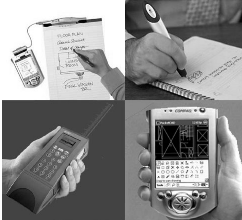
Figure 1. Clockwise from upper left: Seiko Inklink used with iPaq and a notepad, Logitech Io with special notepad, Compaq iPaq, and Leica Disto. (Photos from manufacturers' web sites.)
