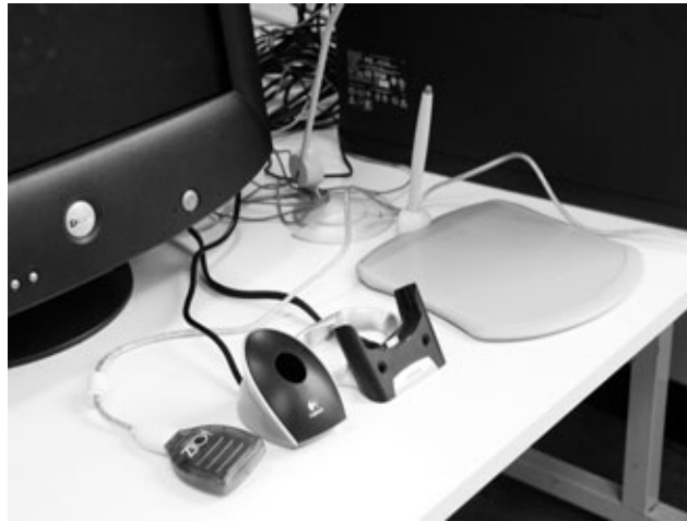
Figure 4. Cradles for transferring information lead to traffic jams at the computer. From the left: Zio memory card reader, Io Pen cradle, iPaq PDA cradle, and Wacom mouse tablet.
