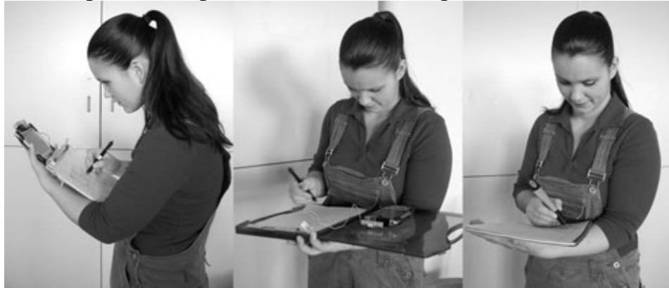
Figure 2. Some tools are easier to use than others. At left, the Inklink connects to the iPaq with a tiny cable and to a notepad with a clip, all hard to hold while sketching. By using a plastic file folder to hold the tools, center, the devices are slightly easier to use. On the right, the standalone Io pen can be used like a normal pen with a special notepad.
