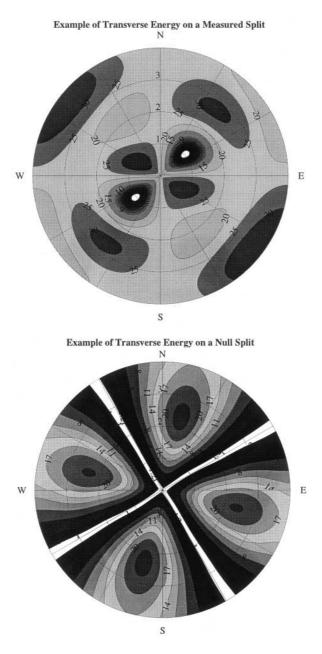
Plots of transverse energy as a function of fast axis orientation and split time. The minimum corrected energy gives the maximum likelihood split parameters. Radial distance is split time in seconds and angle is orientation of the fast axis. Energy levels are in relative units, normalized so that the 95% confidence bounds are indicated by the white area. (Top) Example for a split arrival. (Bottom) Example for a null split arrival.
