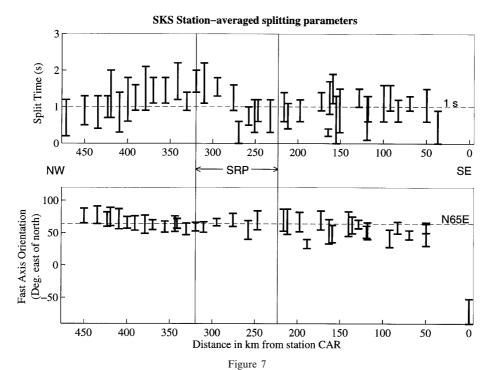
Station-averaged splitting results, obtained from the *F*-test results derived from plots exemplified by Figure 5. A depression in split time is seen, centered southeast of the axis of the Snake River Plain (SRP). Results with major errors have not been plotted: total  $\delta t_{\rm err} > 1.4$  s or total  $\phi_{\rm err} > 40^{\circ}$  (all results tabulated in Table 2).
