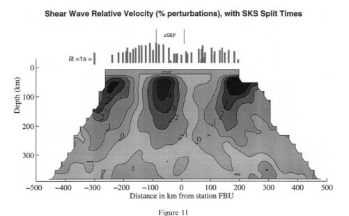
Upper mantle shear-wave velocity and station-averaged split times. (Split times with  $\delta t_{err} > 1.4$  s are not shown). The depression in split times appears not to correlate with velocity structure. However, because all split determinations are derived from arrivals emanating from the NW, it is possible that the offset pattern is a result of being projected to the SE.
