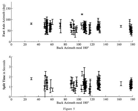
Split parameters with event back azimuth mod 180, using data from Table 1 ( $\delta t_{\rm err} < 0.5$  s). We have excluded the event with  $\delta t = 4.0$  s. Error bars show the calculated 95% confidence intervals. We see no trend with back azimuth, suggesting that splitting occurs near our array. Actual distribution of back azimuths is void of events with back azimuths from the southeast hemisphere.
