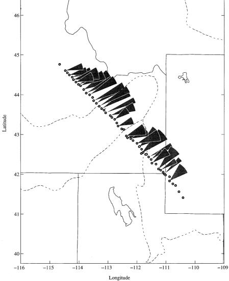
Station-averaged splits plotted in a map view. Width of each sector indicates approximate 95%confidence bounds in orientation of the fast axis. Split times range from 0.3-1.5 s (confidence bounds are not shown for clarity). Station averages with total  $\delta t_{\rm err} > 1.4$  s or  $\phi_{\rm err} > 40^\circ$  are not shown. Fast axis orientations to stations in the northwest appear to be systematically rotated with respect to the other stations.
